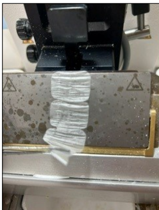
At left is a ribbon of tissue sections coming out of a machine. The ribbon is then put in a water bath, and then one by one each section is picked up on a slide.
