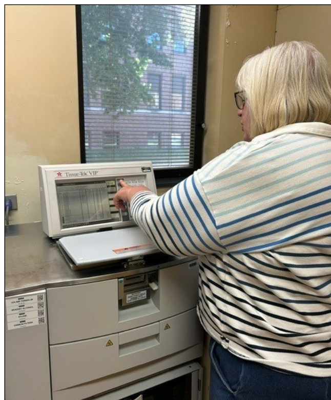
Above is a cross-section of muscle tissue collected from the longissimus dorsi muscle, essentially the ribeye. At right, Ginny uses the tissue processor, which infiltrates a specimen with wax.
