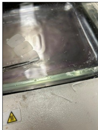
At left is a ribbon of tissue sections coming out of a machine. The ribbon is then put in a water bath, and then one by one each section is picked up on a slide.
