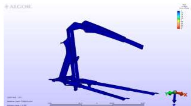
Figure 5.25. Final design FEA factor of safety result with forward load on beam.
