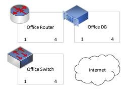
In the top row, a router and rack-mounted server are shown. The second row shows a switch and the internet cloud. The use of these devices to create a basic network, that could be a single internet-connected subnet in CRPG, is shown below.
