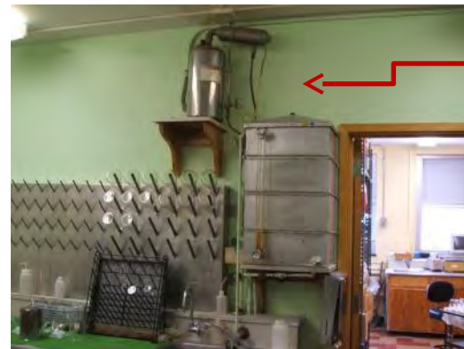
Portable, makeshift water distiller/storage
