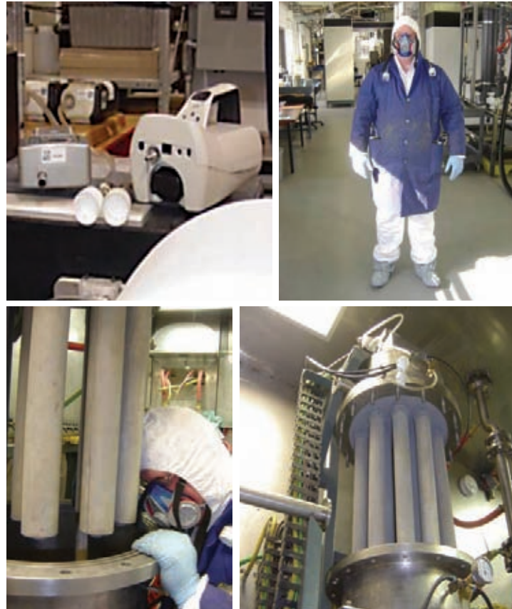
Figure 1. A demonstration of the initial assessment technique with side-by-side sampling using (from left to right) the OPC, co-located open-face filter cassettes, and the CPC: examples of PBZ and source-specific filter-based sampling setup.
