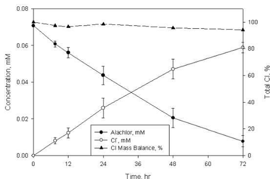
**Figure 4:**  $\text{Cl}^-$  evolution during alachlor degradation. Iron mass loading:  $4 \text{ g L}^{-1}$ . Error bars represent  $\pm$  standard error. Dotted line represents the percentage of  $\text{Cl}^-$  (alachlor +  $\text{Cl}^-$ ) recovered in IC and HPLC analyses.
