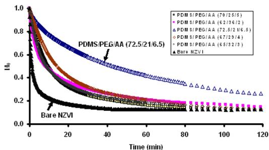
**Figure 7.** Sedimentation studies of APGC coated nZVI (PEG = polyethylene glycol and AA = acrylic acid). Ratio represents weight percent of each component. Marked decrease in sedimentation rate was observed for APGC modified nZVI as compared to bare nZVI.
