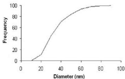
**Figure 5b.** Size distribution curve for synthesized nZVI
