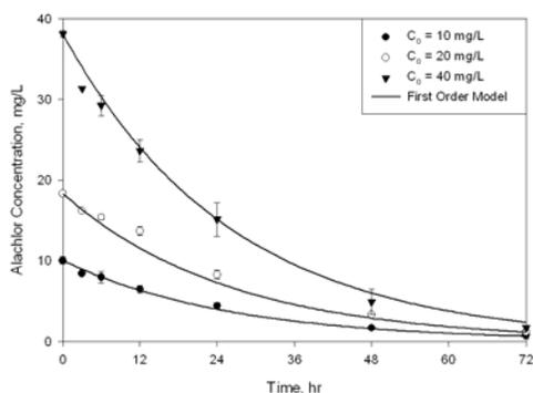
**Figure 3:** Alachlor degradation and modeling results in the presence of nZVI at differing initial concentrations. Iron mass loading:  $4 \text{ g L}^{-1}$ . Error bars represent  $\pm$  standard error. Controls (not shown) do not display appreciable alachlor degradation.
