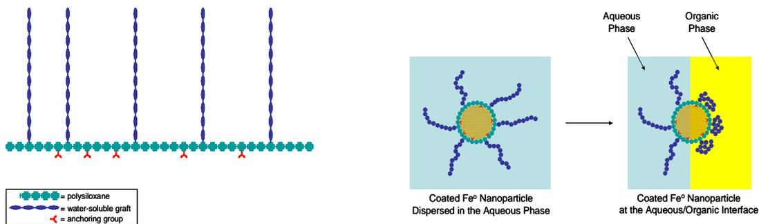
**Figure 1.** A schematic representation of amphiphilic polysiloxane graft copolymers (APGC) **Figure 2.** A schematic representation of the polymer coated nanoparticles in water and at the water/contaminant interface.
