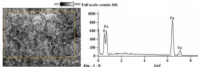
**Figure 6.** SEM/EDX image of fresh nZVI synthesized in the laboratory. The EDX result indicates 84.34 %iron and 15.66 %oxygen on nZVI.
