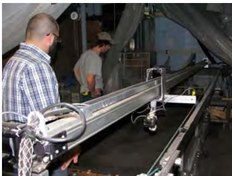
**P2P Experiments (laser scanner and rainfall simulator)**
